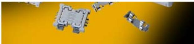
The 9609 Series LED backlight connectors are single-pin, board-to-board style connectors that can be mounted on the outside of lighting strips to provide a higher density of LEDs on the PCB. The design and mounting process is aided by the availability of similarly shaped receptacle connectors in both joint and wire-to-board styles.
