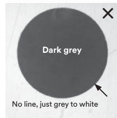
Fiber is missing, cut off connector. Go to step 3 with new connector and restart the termination process.
