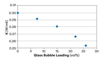
Figure 5. Thermal conductivity as a function of glass bubble loading
