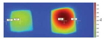
Figure 4. Cooling from the melt with (left) and without (right) glass bubbles
