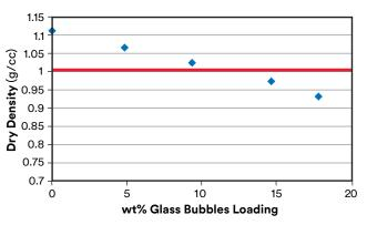
Figure 1. Density of HDPE/Wood composites as a function of GB loading
