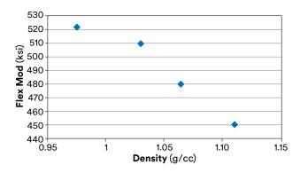
Figure 3. Flexural Modulus as a function of density
