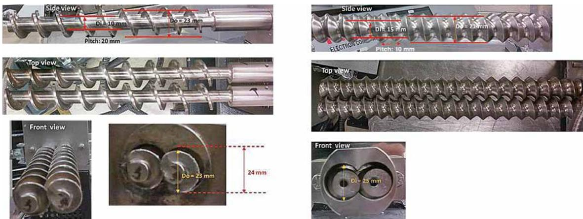
**Figure 9.** Auger configuration for the glass bubbles side feeder (left) and supply feeder (right)
