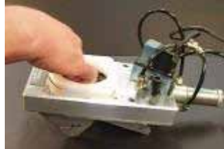
Remove the white plastic insert from the main frame.
