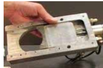
Clean and inspect the shoe. Reassemble in reverse order.
