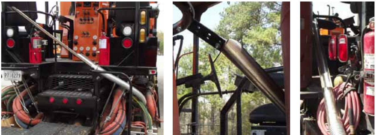
Figure 7: Securing feed tube and flex tube
