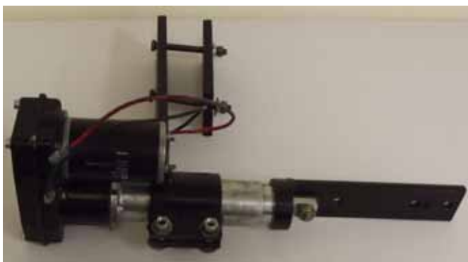
Figure 6: "O" Bracket Mounting with Linear Actuator
