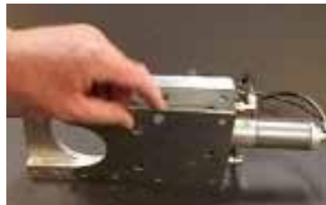
Remove the wear plate from the main
