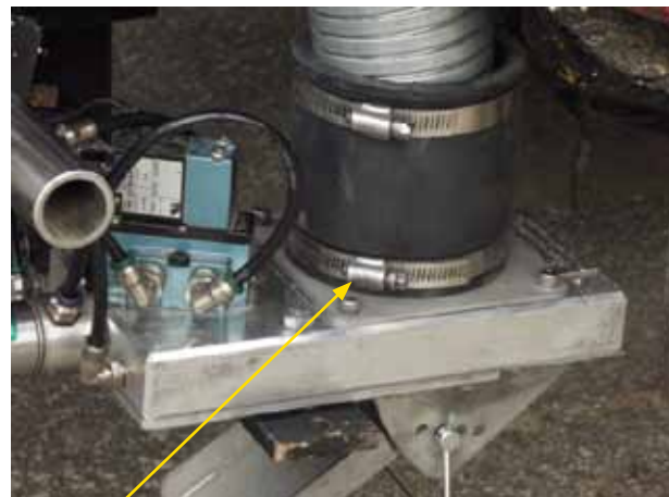
Remove the end of the flex hose from the funnel, add the flexible coupling, and reseat the flex hose.
