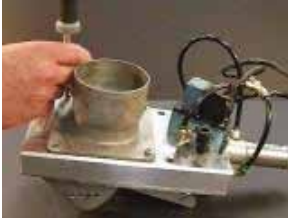
Remove the external cap screws on the feed funnel.
