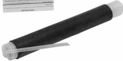
They are factory expanded and assembled onto a core which is removed after the tube has been positioned for installation over an inline connection or harness section. The tube shrinks, forming a dynamic, environmental seal which resists prolonged aging and exposure. It installs quickly with little training and no tools or heat source.
