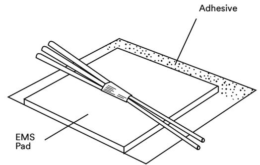
**NOTE:** Do not hold wires while compressing pad. Hydraulic pressure from compressed adhesive will flair the wires automatically causing the adhesive to flow between and seal the wires. Pressed pads may be reshaped to make the covered junction more compact.
