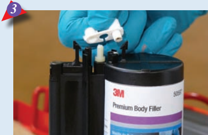
3 Remove sealing cap from Premium Body Filler (50597/50598) . Attach Dynamic Mixing System Nozzle 50601
