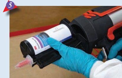
5 Turn the Dynamic Mixing System Applicator 50600 air regulator 2.5-3 turns clockwise (from a closed position)
