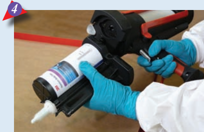
4 Align the Premium Body Filler (50597/50598) with the Dynamic Mixing System Applicator and twist into place.
