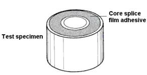
Outer and inner tubes: 230 mm long tubes, aluminium alloy 5052-0 bare. Outer tube: diameter 25.0 mm, thickness 1.25 mm. Inner tube: diameter 12.5 mm, thickness 1.25 mm.
