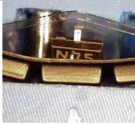
Rework (at peel enabling feature on 3M™ Universal Cover (UCT) Tape 2688A
