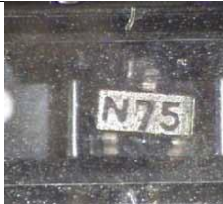
Rework (resealed) on 3M™ Universal Cover (UCT) Tape 2688A
