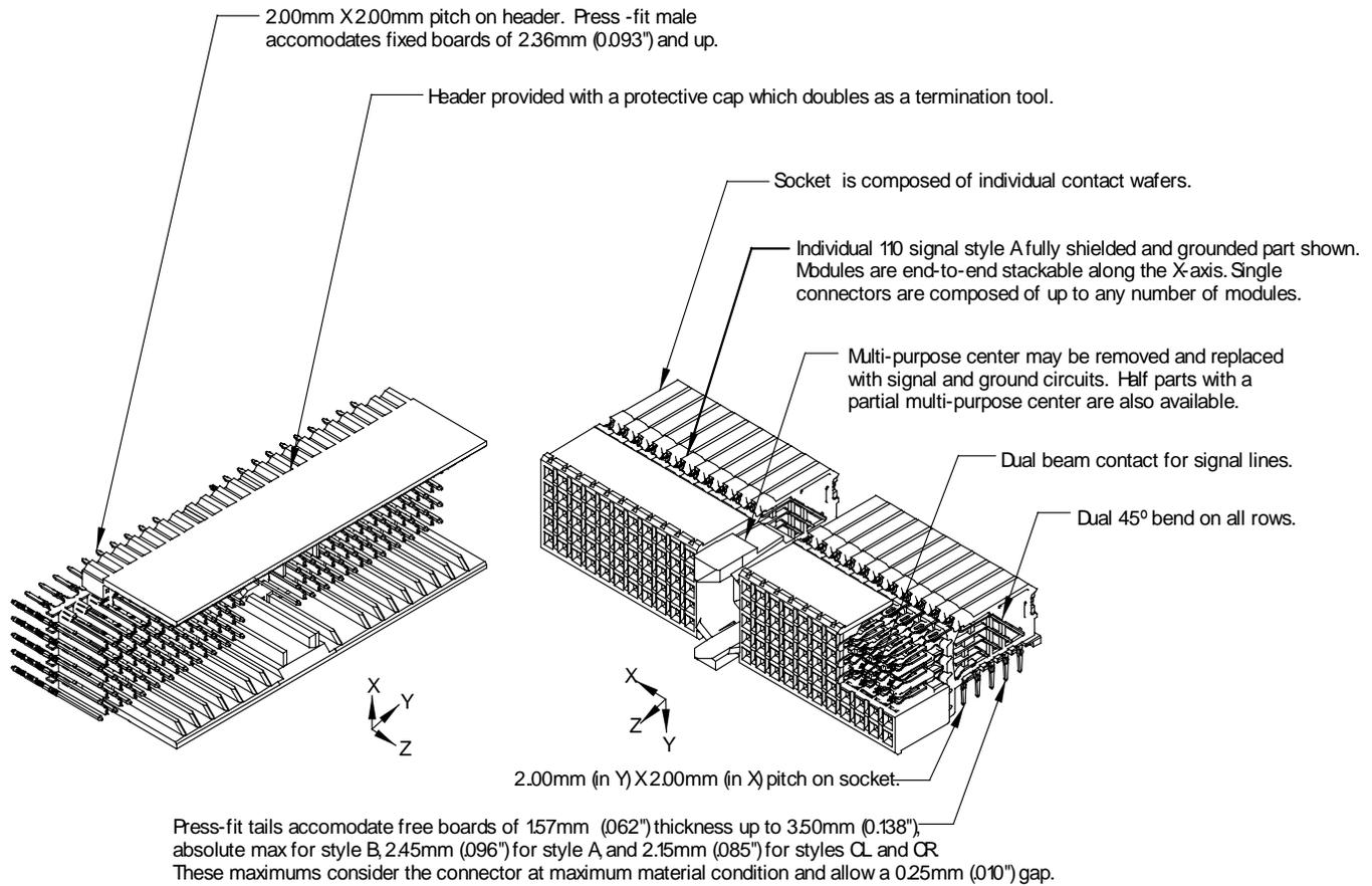
Note: For more detail see the module specific tech sheet. Board thickness of plus or minus 10% of the shown nominal is acceptable. Socket board thickness greater than those called out above are possible but require special notching and or chamfering (see section 4.2.A).
