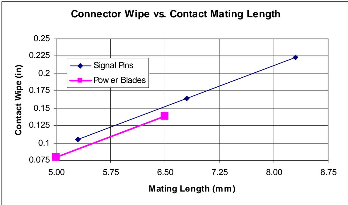
Note: Shield mate length and wipe are constant, 4.50mm (0.177") 1.60mm (0.063") respectively.
