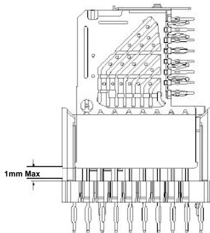
Note: Electrical performance will be impacted due to the under-seated gap. Contact 3M Engineering for specific information.
