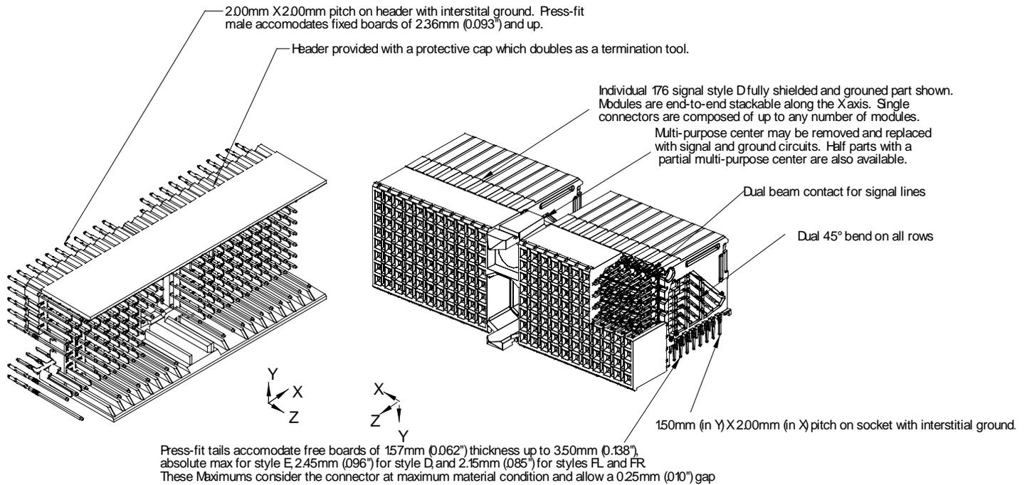
Note: For more detail see the module specific tech sheet. Board thickness of plus or minus 10% of the shown nominal is acceptable. Socket board thickness greater than those called out above are possible but require special notching and or chamfering.
