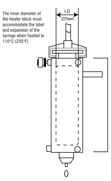
The heater block should extend the full length of the syringe to just under the attachment of the pressure cap
