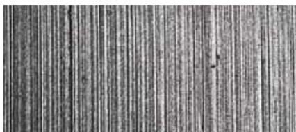
Magnified view of straight line finished surface
