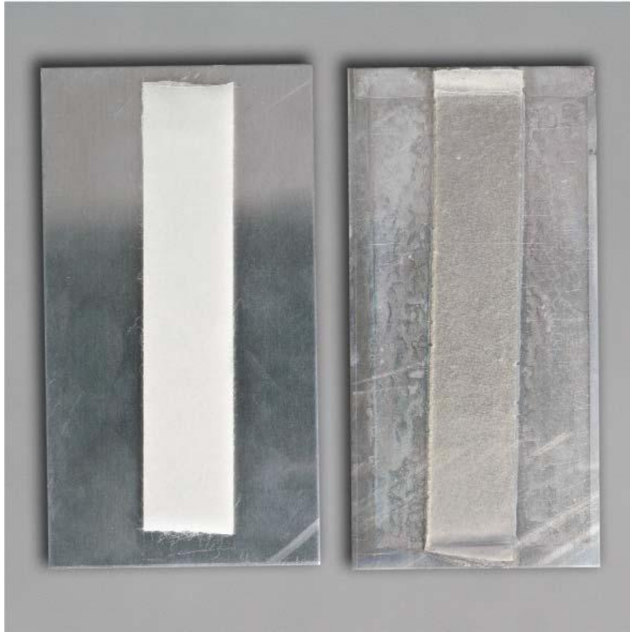
Visual comparison of freshly applied 3M™ Extreme Sealing Tape 4412N (left); and 3M™ Extreme Sealing Tape 4412N after weathering in direct UV exposure.
