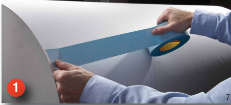
1 Apply tape beginning and ending 1/4" from edges.
