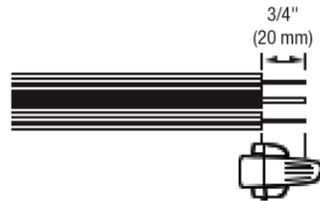
2. With wire ends even, insert wires into the connector and tighten until secure.
