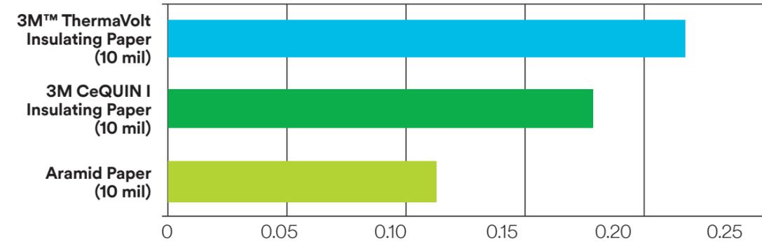
Thermal conductivity (W/mK) tested per ASTM E-1530 @ 180° C
