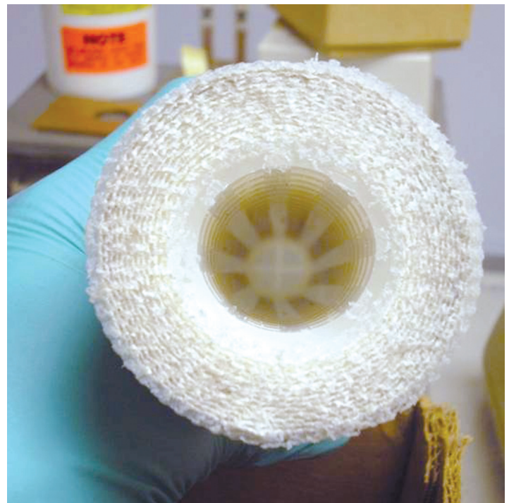
3A. Cross section of Returned 3M™ Betapure™ NT-T Series Cartridge – note penetration of D.E. fines into the media pack of the filter
