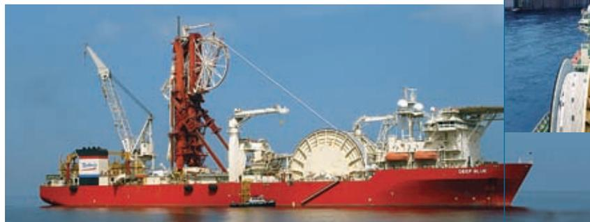
Deep Blue: Technip's deepwater pipelay vessel
