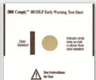
Indicator circle on Early Warning Test Sheet does not match color standard and Bowie-Dick test sheet shows a non-uniform color change. Test sheet result indicates a small amount of residual air in the chamber.
