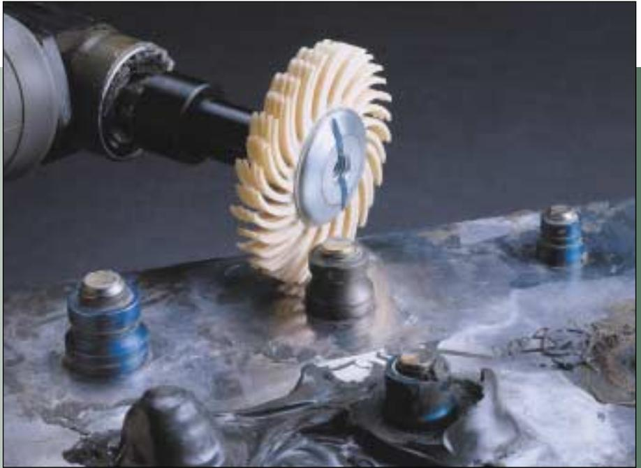
2" SR Radial Bristle Disc cleaning final layer of seam sealant around aircraft fuel tank fasteners.
