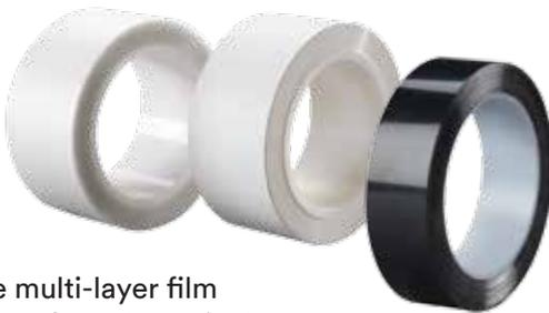
3M™ EPE Films are multi-layer film products consisting of ethylene vinyl acetate (EVA) layers bonded to both sides of a polyester film. They can be used with crystalline silicon and thin-film solar cells in rigid and flexible modules. Applications include providing electrical insulation between components and serving as a cosmetic mask to provide consistent appearance.
