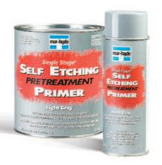
Mar-Hyde® SINGLE STAGE® SELF-ETCHING PRIMER is a ready-to-spray, pretreatment/primer that provides excellent corrosion protection and creates a superior bond to most metals by chemically etching the surface of the panel. It is solvent resistant, has excellent adhesion to aluminum, bare steel, galvanized steel and fiberglass and can be topcoated with all automotive primers and paint systems. Ready-to-spray VOC of 6.4 lb/qal. USEPA National Rule and California Rule 1151 compliant.
