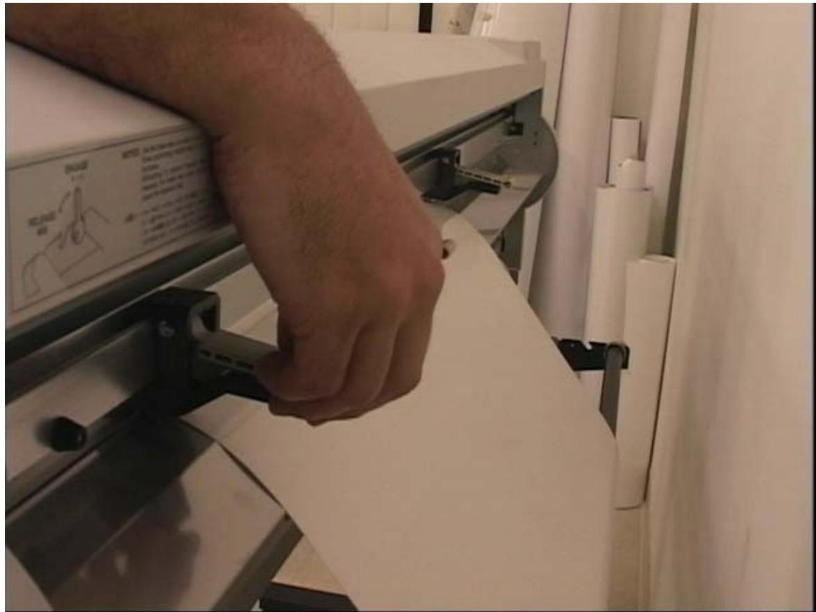
6. Raise the pinch rollers, and then feed the media under the pinch rollers.
