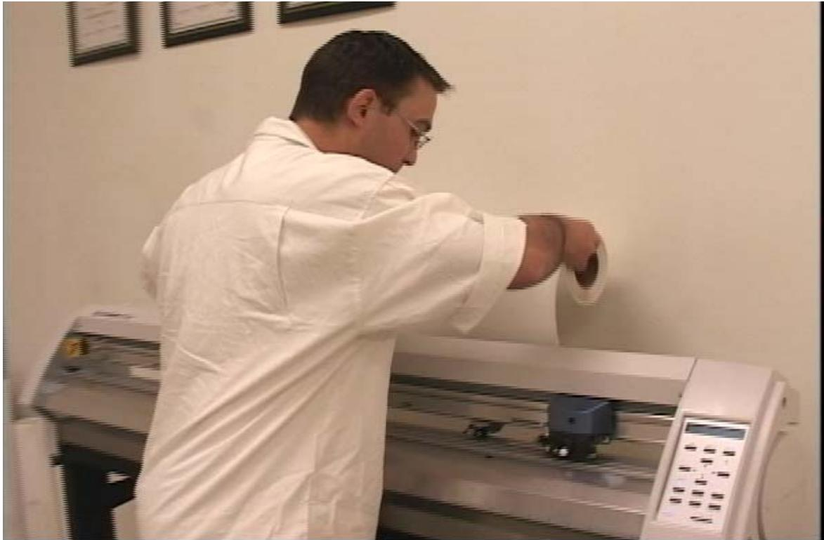
5. Behind the plotter are levers that are used to raise and lower the pinch rollers when loading media.
