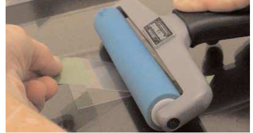
Figure 4. Rolling down the OCA/CEF.
