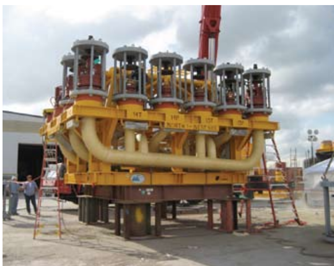
Cuming Corp. C-THERM epoxy syntactic foam thermal insulation applied to a BP Atlantis subsea production manifold. Photo courtesy of Cuming Corp.
