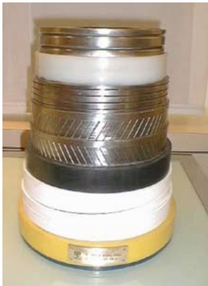
Technip insulated flexible pipe sample wrapped with syntactic tape layers. Photo courtesy of Technip.
