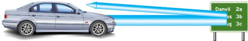
**3M™ Diamond Grade™ DG<sup>3</sup> Reflective Sheeting, made with 3M Full Cube Technology, reflects 58% of light back toward its source—almost doubling the overall brightness of road signs.**
