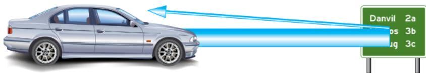
**One of the original retroreflective technologies, encapsulated glass bead sheeting reflects only 14% of light back toward its source.**
