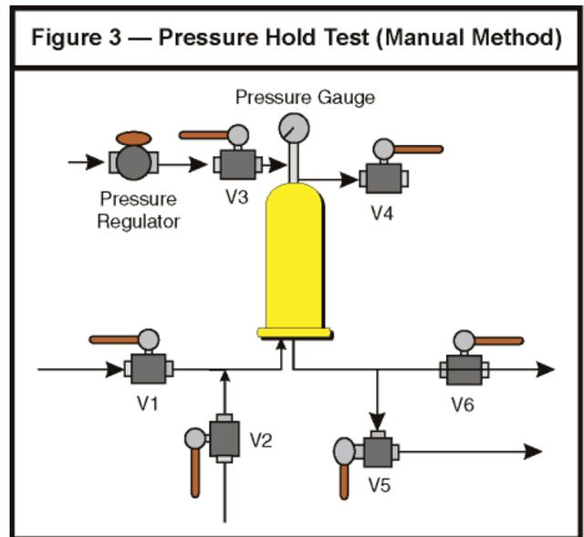
\* Use of CO<sub>2</sub> in the integrity test will result in a false reading.
