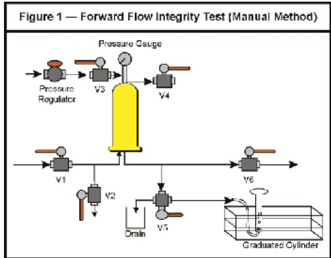
3. Adjust either the downstream valve V6 or the drain valve V5 to restrict the flow of water and apply a back pressure on the housing.
