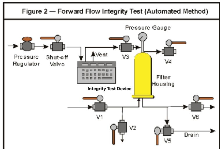
\* Use of CO<sub>2</sub> in the integrity test will result in a false reading.
