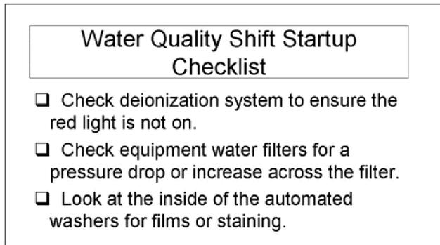
in the department understand what the alarm indicates. A worker could assume the red light on a DI system indicates the system has power and allow the decontamination process to continue with a failed purification system. Even looking at the inside of the washing equipment and examining the instrumentation can be used as a way to monitor water impurities. If a sterile processing professional knows the signs
