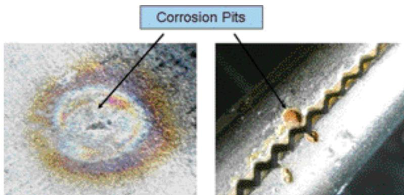
These pits can harbor soil and microorganisms during reprocessing and sterilization.<sup>2</sup> Pits can also weaken and jeopardize the functionality of instrumentation.
