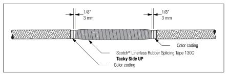
Apply two highly-stretched half-lapped layers of 13 tape over the 130C tape
