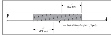
7.5 Starting 1" (25 mm) past the 31 tape, apply 3 half-lapped layers of 1700P tape to each end to temporarily secure the ends of the 31 tape until the tape reaches full bond.
