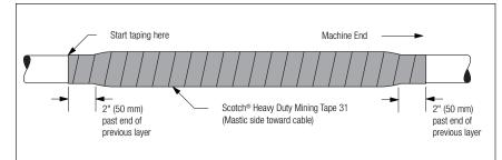
5.3 Starting 1" (25 mm) past the 31 tape, apply 3 half-lapped layers of 1700P tape to each end to temporarily secure the ends of the 31 tape jacket until the jacket reaches full bond.
