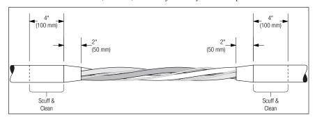
6.5 Wrap half-lapped layers of 130C tape (**tacky side DOWN**) building up and across the splice until equal to or greater than original jacket thickness and extends 1" (25 mm) past the top of jacket tapers.
