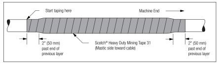
6.7 Starting 1" (25 mm) past the 31 tape, apply 3 half-lapped layers of 1700P tape to each end to temporarily secure the ends of the 31 tape until the tape reaches full bond.
