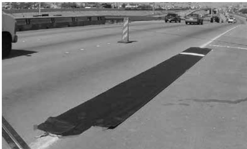
Figure 2. Tar paper layout for test line application.
