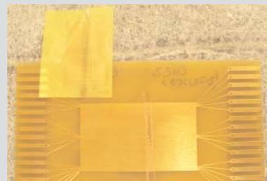
**Figure 9. Residual ACF in Bond Area.**
