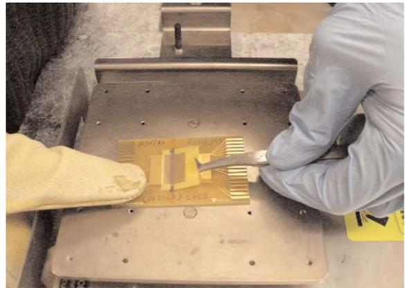
**Figure 4. Debonding Using Hot Plate.**
