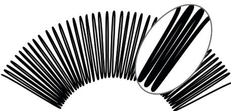
Conventional pleat designs, with full-depth densely packed pleats, fill the upstream pleat surface with contaminant that quickly constrict flow at the pleat's inside diameter.
