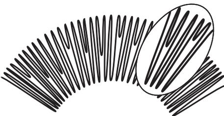
The 3M™ Betafine™ XL series filter cartridge's Advanced Pleat Technology utilizes a configuration designed to increase the accessible surface area for significantly greater filter media use.
