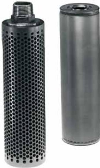
CUNO™ metal screen filter elements are produced from premium quality woven stainless steel screen mesh. Elements are all 304 or 316 stainless steel, with screen and perforated internal support attached to end caps equipped with replaceable gaskets. Elements can be cleaned chemically or ultrasonically and reused. Cylindrical elements may also be cleaned in place by backflushing. Request literature LITMSPKCLN for recommended cleaning instructions.
