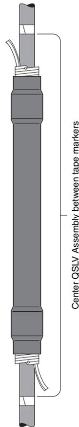
5. Pull one of the loose pull tabs while unwinding (counter-clockwise) to lock 3M™ Cold Shrink Insulator QSLV-M into place. Pull the other loose pull tab while unwinding (counter-clockwise). Installation is now complete.
