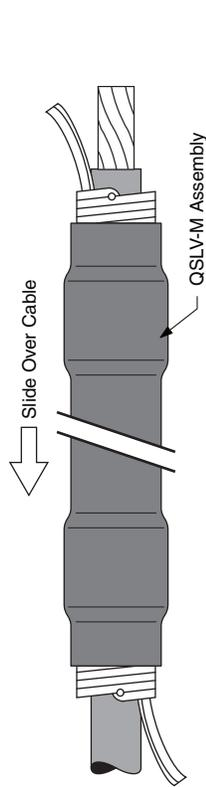
2. Make connection. Place a tape marker 7" (180 mm) from the center of the crimped connector on both Cable A and Cable B sides.
