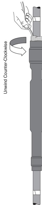
**Note:** The ends of the 3M Cold Shrink QSLV-M Insulator may be squeezed to assist the tube in shrinking to its final diameter.
