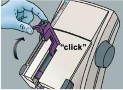
Fig. 9 Locking lever snaps into the uppermost position.
