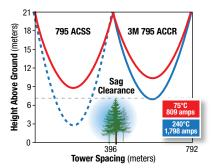
Actual performance may vary depending on a number of variables. The example above assumes ACSS and 3M<sup>™</sup> ACCR with a 396 m. ruling span under the following conditions:
