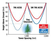
Actual performance may vary depending on a number of variables. The example above assumes ACSS and  $3M^{\text{TM}}$  ACCR with a 1,300 ft. ruling span under the following conditions:
