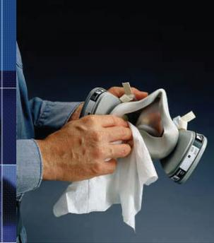
*The proper cleaning and maintenance of respirators is an important area that is commonly overlooked. All respiratory protection equipment needs to be in good condition to work effectively and to be able to supply the level of protection expected by the user.*
