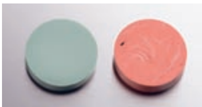
Fig. 6. Superior mixing quality of Express™ 2 Penta™ Putty with the Pentamix™ Mixing Unit (left) compared with a putty mixed by hand (right, Express STD Putty).
