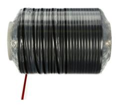
3M™ Acrylic *Plus* Tape WT4100 Series tapes are acrylic foam tapes, constructed with two different adhesives, and are available in two thicknesses – 0.8 mm and 1.2 mm. These tapes are typically used to attach weatherstrip and/or gasket seals for automotive and industrial applications, such as sunroof seals, lamp seals, and taped seals on the vehicle door.
