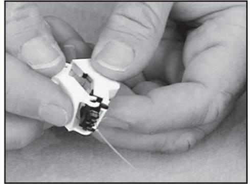
Rotate the base on the housing until the housing and base latch closed with an audible click.
