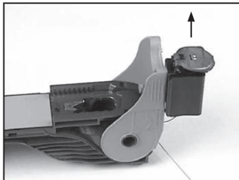
Place the polishing puck assembly into the scribe entrance by inserting the exposed fibers into the fiber stub basin.
