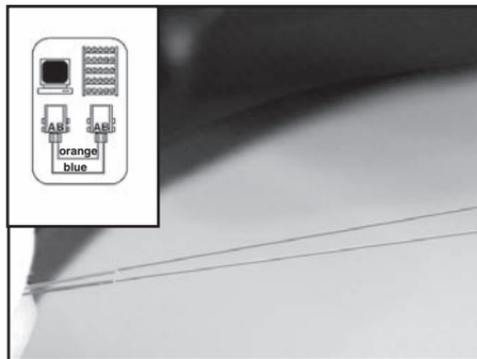
**Slide the fibers along the fiber guide grooves** of the polishing puck assembly and into the socket fiber holder.
