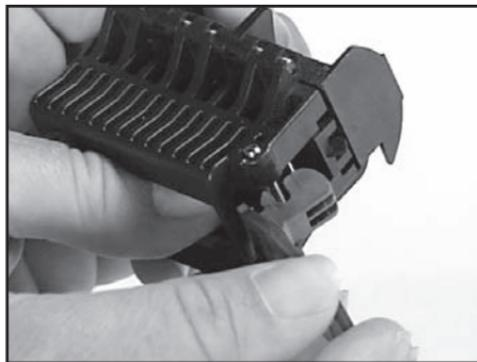
5.5 **Clean the fiber guide holes of the polishing face.**
