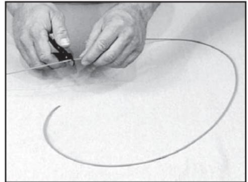
Remove the outer sheath by pulling on the end of the cable jacket, sliding it off the Kevlar® strands and inner optical fiber buffer tubes. Do not use the tool to slide the outer jacket off the inner Kevlar strands and buffer tubes. Discard the outer jacket.
