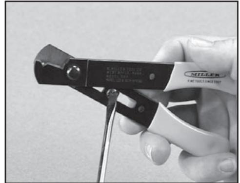
4.5 **Remove outer cable sheath.**
