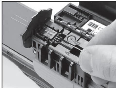
**Place the buffer tube into the strain relief foam** so that the two fibers are held with a slight bow in the socket fiber holder.
