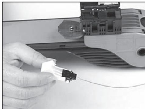
Hold the base and align the base “hinge” over the pins of the housing. Snap the “hinge” over the “pins.”
