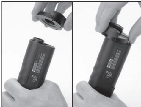
Insert the polishing puck into the puck adapter. An audible click will be heard when the puck is fully seated. (Note: the adapter is keyed to accept the puck in only one direction).
