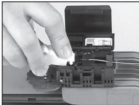
Remove the housing from the polishing puck assembly (the fiber holder will be attached to the housing).
