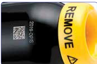
Figure 1. Laser Etch 2D Barcode
