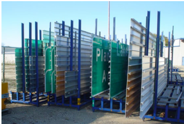
Figure 5. Extruded signs shown secured vertically for temporary outdoor storage.
