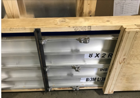
Figure 4. Large sign storage. Each crate contains two signs of similar size that have been secured to maintain an air space between the two sign faces and eliminate the need for slipsheeting.
