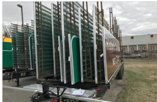
Figure 9. Extruded panel signs secured for transportation. Signs are shown secured vertically, in racks with sufficient space between them to prevent face damage through contact and to facilitate air flow.
