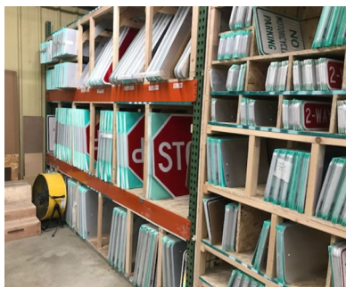
Figure 3. Signs stored vertically on shelving designed to accommodate small signs.
