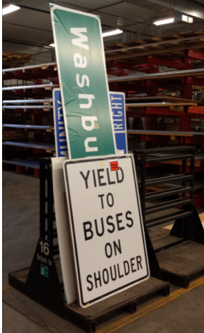
Figure 1. Signs stored vertically on a pallet stand.
