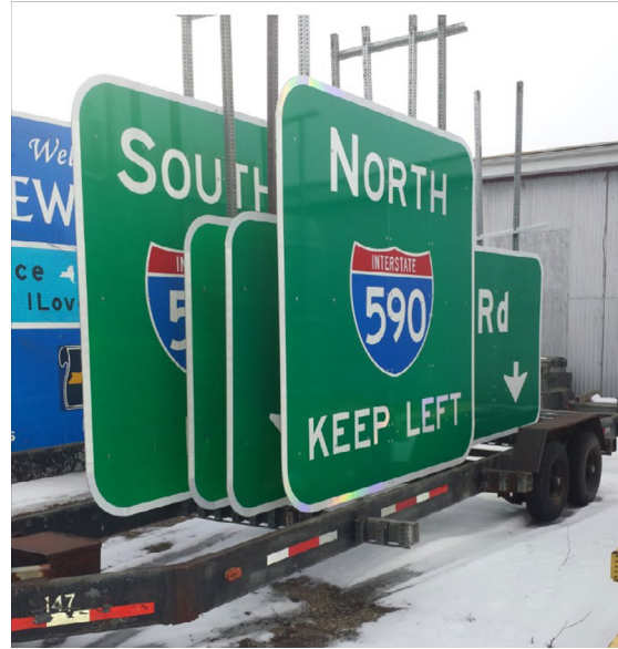
Figure 10. Flat panel signs secured for transportation. Signs are shown secured vertically, in racks with sufficient space between them to prevent face damage through contact and to facilitate air flow.
