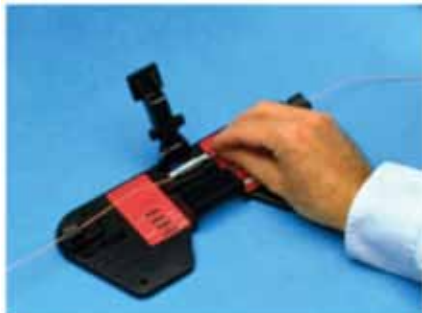
Figure 2 – A mechanical splice activation tool holds the fiber ends in contact and presses the metal element over fiber ends to complete the splice. No power source is required.
