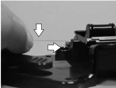
4. Insert the fiber into the splice until it stops.
