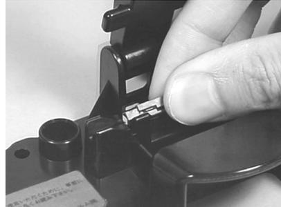
2. Put Fibrlok splice in the tool with the Fibrlok cap up. Strip 30–40mm of fiber buffer and clean the fiber with lint free wipe and alcohol.
