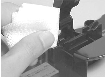
1. Clean both edges of the area where the splice is set in the tool with a lint free wipe and alcohol.
