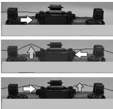
7. Hold down the arm where the second fiber will be inserted. Insert the second fiber until the first fiber bows as shown. Release the arm and push the first fiber to equalize the fiber bows as shown.
