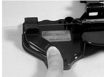
5. Press arm down and place fiber into open foam holder. Release arm so that the foam holder retains the fiber.
