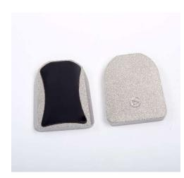
3M™ Structural Bonding Tapes (SBT) 9214 and 9263 are formulated for bonding hardware components to glass, such as rearview mirror components, sensor brackets and mounting pins. 3M SBT is applied as a pressure-sensitive tape and then is heat-cured to develop semi-structural strength.
