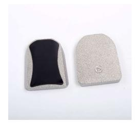
3M<sup>™</sup> Structural Bonding Tape (SBT) 9270 is formulated for bonding hardware components to glass, such as rearview mirror components, sensor brackets and mounting pins. 3M SBT is applied as a pressure-sensitive tape and then is heat-cured to develop semi-structural strength.
