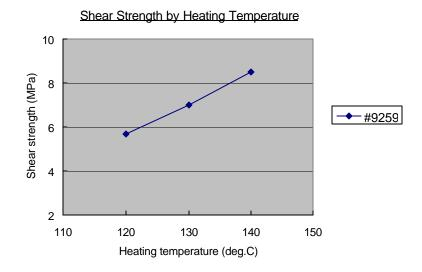
\*Heating condition : 20 min keep in settled temperature conditions.
