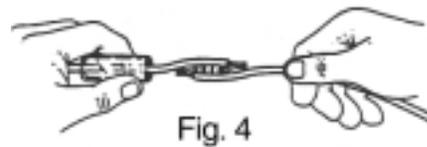
Center the tubing over the component (Fig. 5). With the ST-3000 and ST-3006 infrared heating units this is easily accomplished by placing the welded connection over the small circle on top of the heating chamber, then centering the tubing with respect to the red outline.
