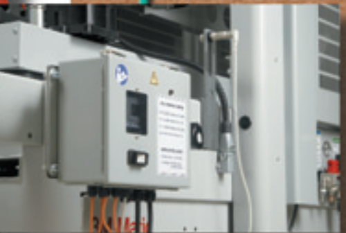
Electrical control box with Programmable Logic Controller (PLC) mounts on side of 3M-Matic™ Case Sealer and displays informational and error codes
